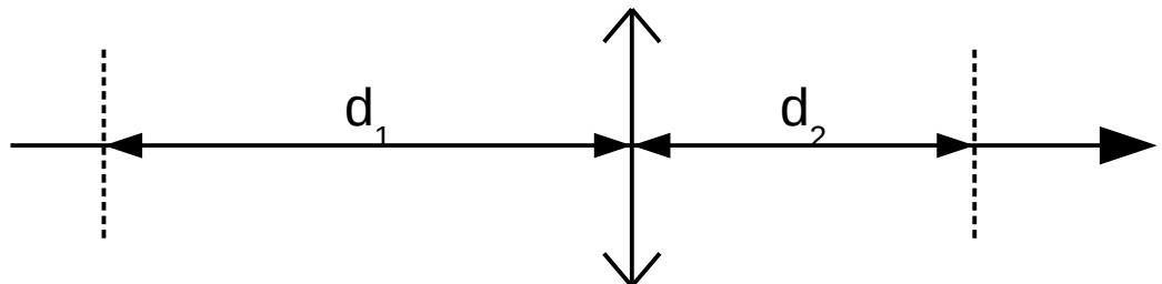
$$\begin{pmatrix} m_{11} & m_{12} \\ m_{21} & m_{22} \end{pmatrix} = \begin{pmatrix} 1 & d_2 \\ 0 & 1 \end{pmatrix} \begin{pmatrix} 1 & 0 \\ F & 1 \end{pmatrix} \begin{pmatrix} 1 & d_1 \\ 0 & 1 \end{pmatrix} = \begin{pmatrix} 1+d_2F & d_1+d_2+d_1d_2F \\ F & 1+d_1F \end{pmatrix}$$
